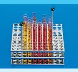
**Test Tube Rack** made of stainless steel, with 100 openings of Ø 18 mm, for test tubes
