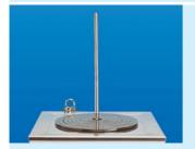
**Support Rod** made of stainless steel, length 316 mm, Ø 12 mm
